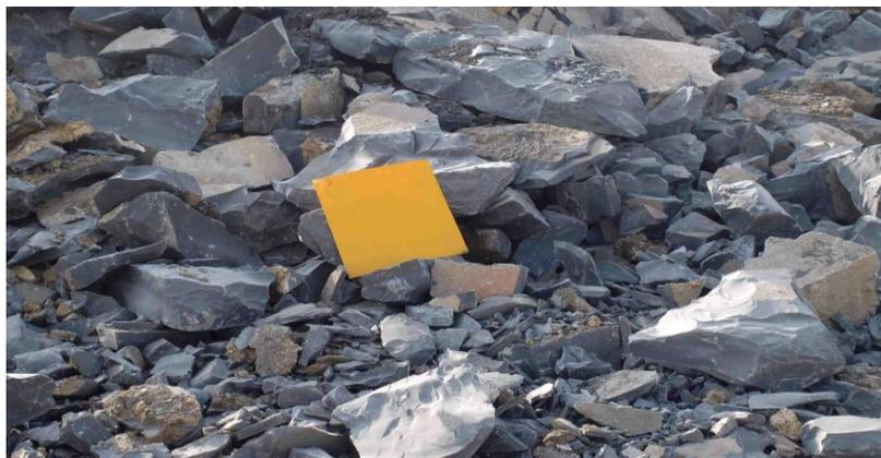
FIG. 13 CALIBRATOR FOR FRAGMENTATION ASSESSMENT USING WIPFRAG
